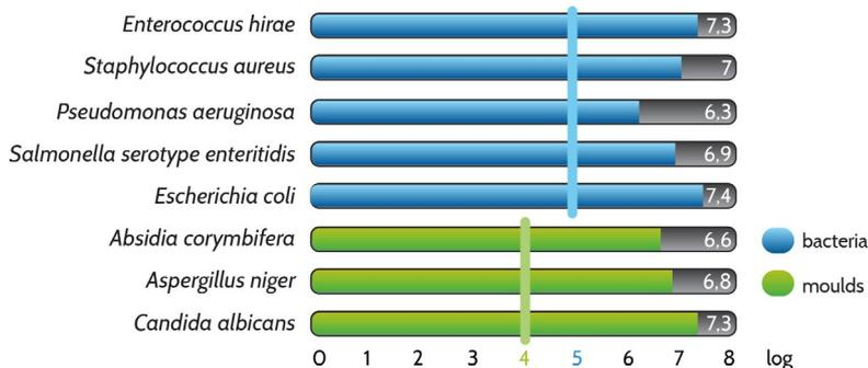
Required efficacy according to standard NF T 72-281: 5 log for bacteria and 4 log for moulds.
